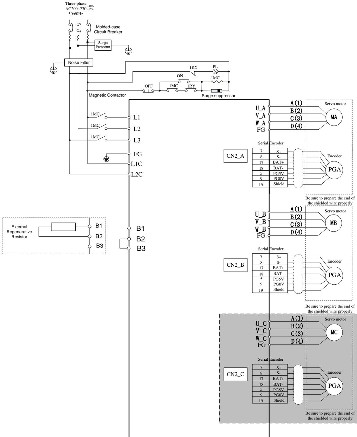
Note :The wiring of ETS two-axis servo drive does not include the gray part of graph.
