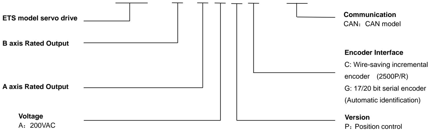
Notes: Each axis of ETS servo drive equips 50W、100W、200W、400W、750W、1.0kW servo motor, and assures three times overload capacity.
