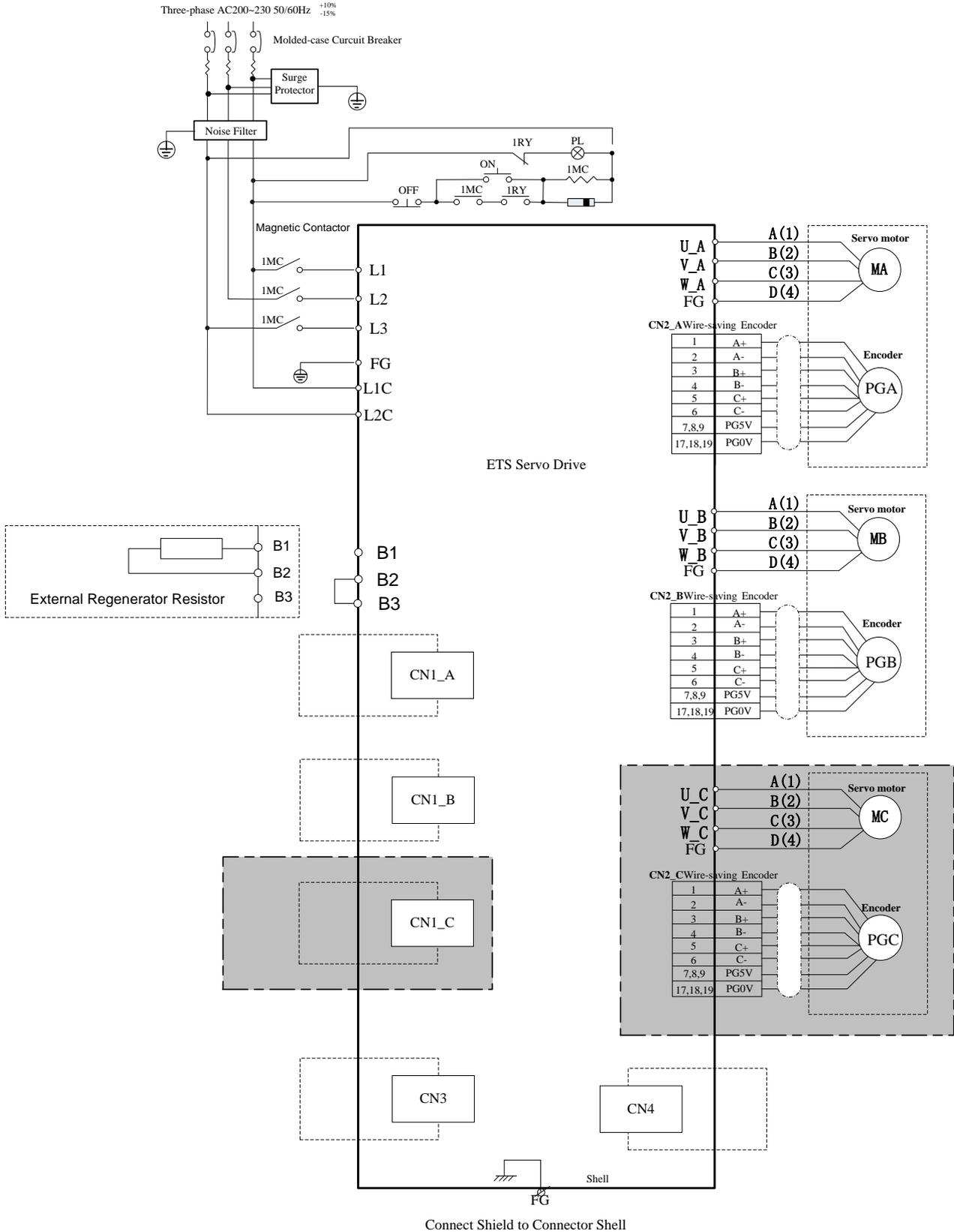
Note :The wiring of ETS two-axis servo drive does not include the gray part of graph.
