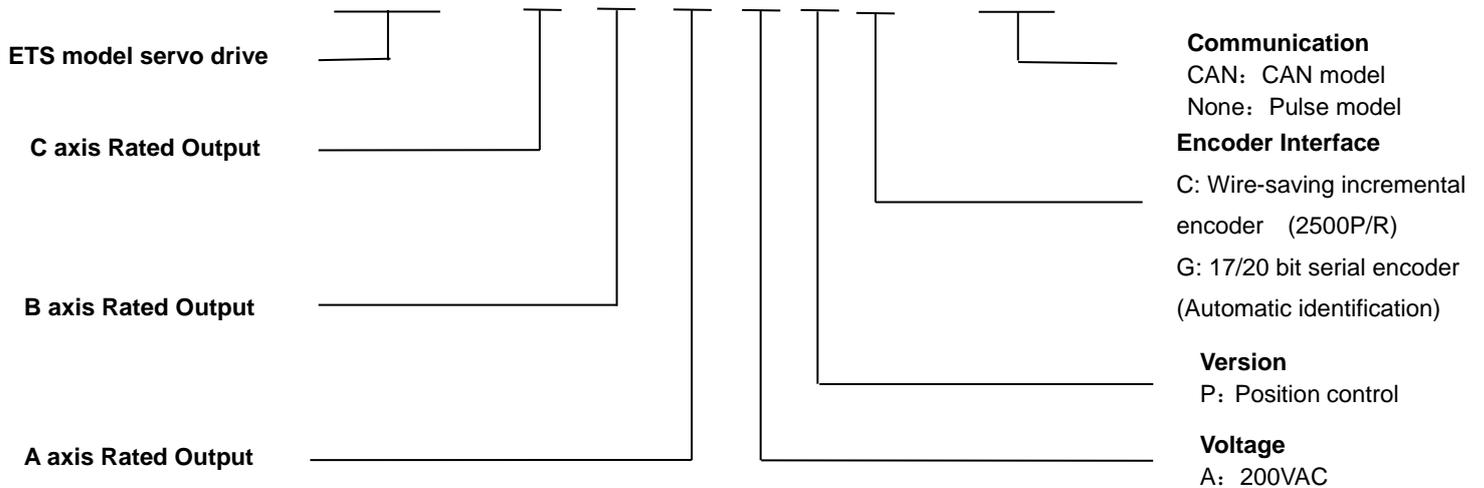
Notes: Each axis of ETS servo drive equips 50W、100W、200W、400W、750W、1.0kW servo motor, and assures three times overload capacity.
