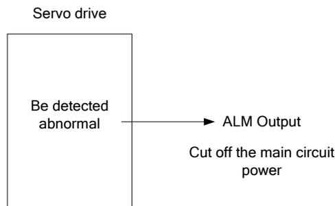
Normally, the external circuit consists of /ALM should be able to switch off the power of servo drive.
