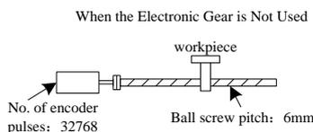
To move a workpiece 10mm :
