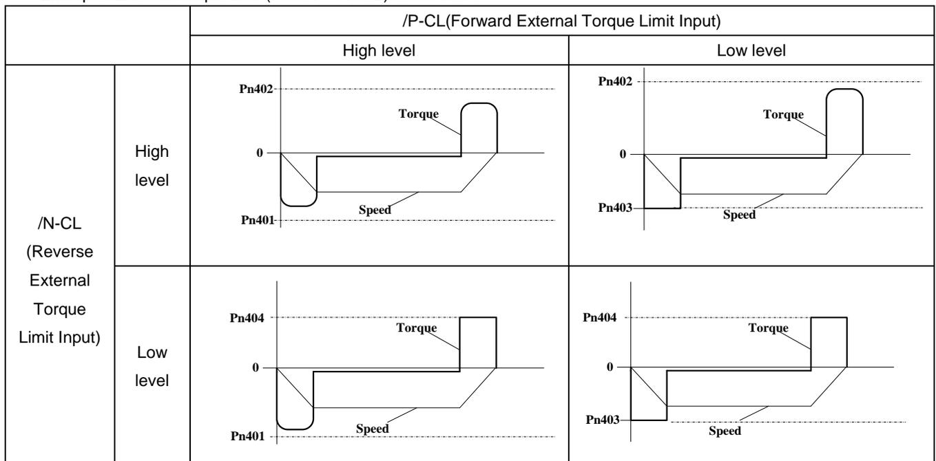
Note: Select the servomotor rotation direction by setting Pn001=b.    0 (standard setting, CCW=Forward direction).
