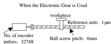
To move a workpiece 10mm using reference units:
