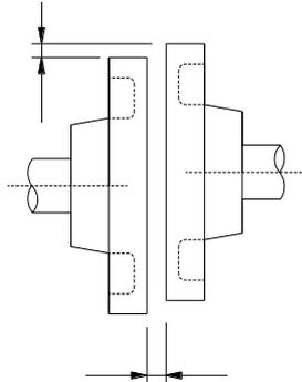
Measure this distance at four different positions in the circumference. The difference between the maximum and minimum measurements must be 0.03mm or less. (Turn together with couplings.)
