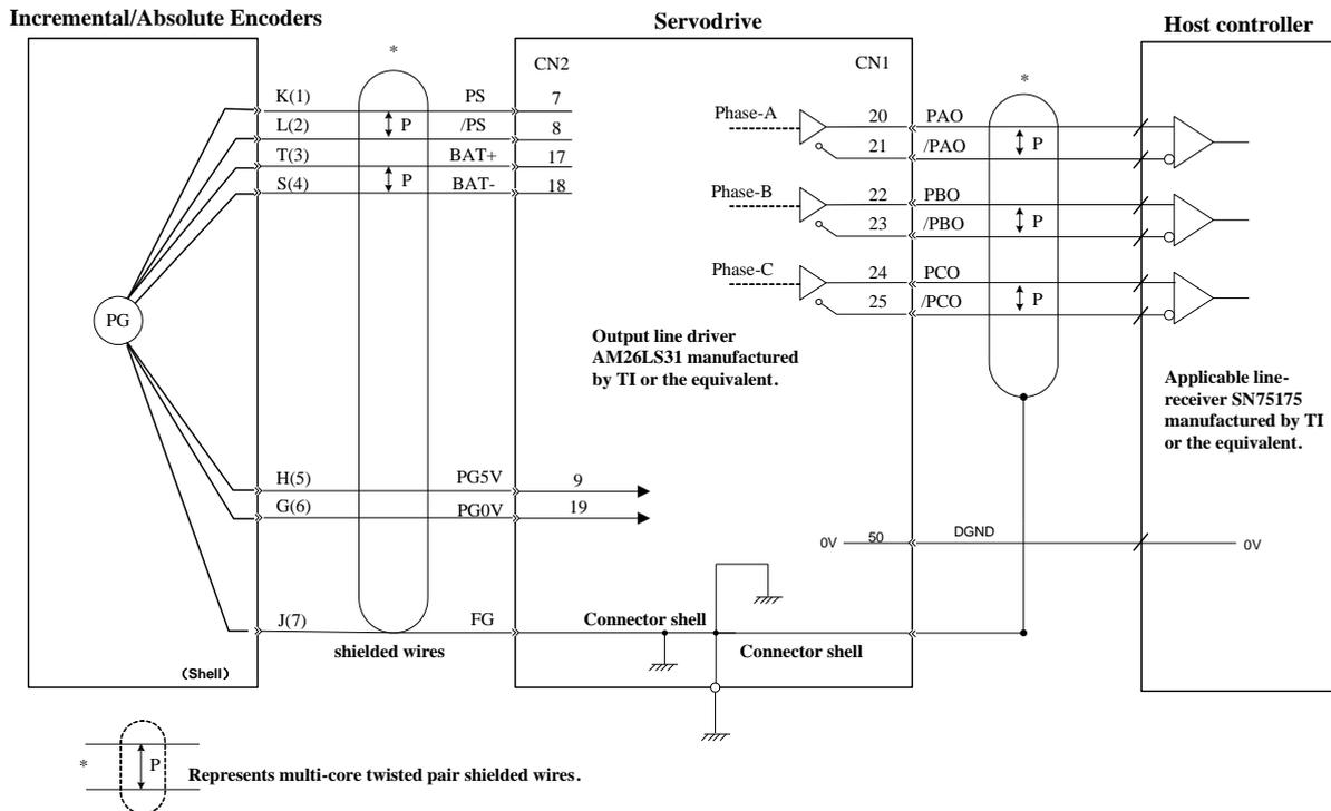
Note: (1)BAT+ and BAT- signals are not used when using an incremental encoder.
