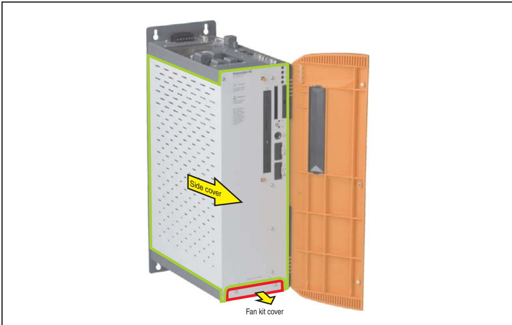
Figure 278: APC620 3PCI slots - Remove side cover and fan kit cover
