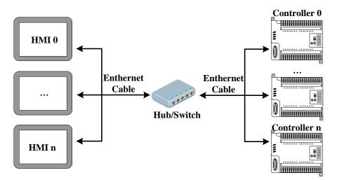
[Examples] Below two MT5320T (hereinafter referred HMI0 and HMI1) and one MODBUS TCP device (hereinafter referred to PLC0), and one OMRON CJ series PLC (hereinafter referred to PLC1) communications as an example. Require to monitor the data of PLC0 4x100 in the HMI0, and to monitor the data of PLC1 D100 in HMI1.
