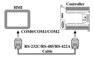
[Example] Below a MT5320T with a SIEMENS S7-200 communication, for example, requires the HMI monitor PLC M0.0 output state. (This example uses the HMI COM0 port to connect PLC communication)
