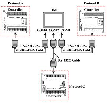
[Example] Below a MT5320T with a SIEMENS S7-200 (hereinafter referred to as PLC 0), a MITSUBISHI FX2N (hereinafter referred to as PLC 1), a OMRON CP1H (hereinafter referred to as PLC 2) communication, for example, Requirements were monitored on the HMI PLC 0 of VW 100, PLC 1 of D100 data and PLC 2 in Q 0.0 outputs.
