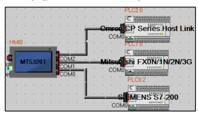
In the [HMI Attribute] - [COM0/COM1/COM2 Setting] According to the serial communications port of the connected PLC actual parameters were set to HMI serial communication parameters, Parameters are set as follows:
