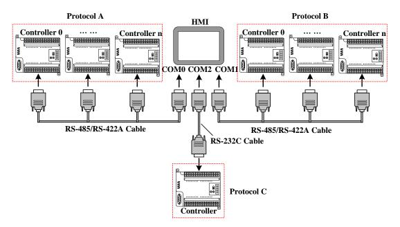
[Example] Below a MT5320T with three MODBUS device (hereinafter referred to as PLC 0, PLC 1, PLC 2), a MITSUBISHI FX2N (hereinafter referred to as PLC 3), a OMRON CP1H (hereinafter referred to as PLC 4) communication is cases, Requirements were monitored on the HMI PLC 0, PLC 1, PLC 2 of 4X 100, PLC 3 of D100 data and PLC 4 of Q 0.0 outputs.
