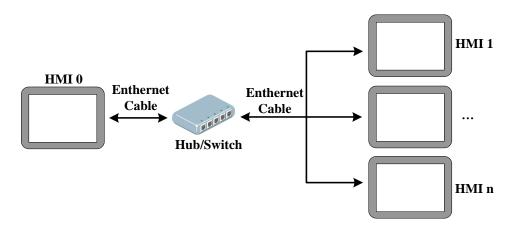
[Example] Below two MT5320T communication, for example, requires HMI0 screen control HMI1 of LB100 status output to ON.
