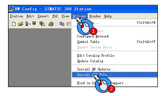
GSD file installed, Right in the HW Config directory PROFIBUS DP / Additional Field Devices / MMI find the appropriate configuration file:
