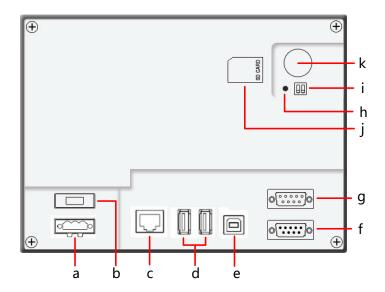
a. Input terminal of power supply DC24V b. 1A Fuse c. LAN interface d. USB HOST(USB type A interface) e. USB SLAVE(USB type B interface) f. COM1(female) g. COM0&COM2(male) h. RESET Button i. DIP Switch j. SD CARD interface k. One-time button type lithium battery
