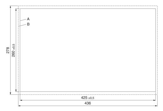
Figure 2-12 Mounting cutout (dimensions in mm)
