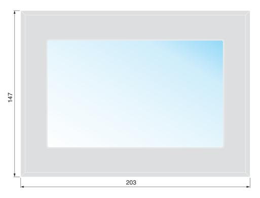
Figure 2-2 Front panel (dimensions in mm)
