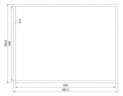
Figure 2-10 Mounting cutout (dimensions in mm)
