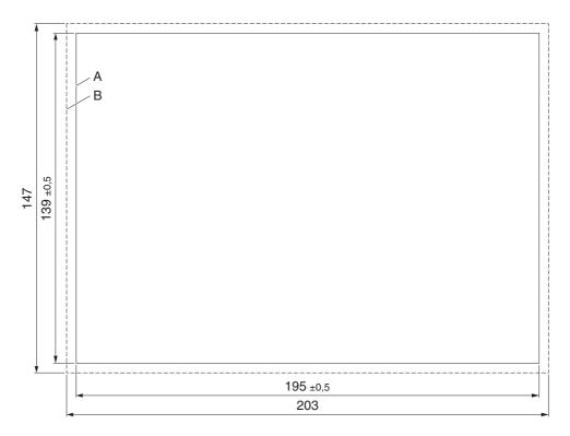
Figure 2-8 Mounting cutout (dimensions in mm)
