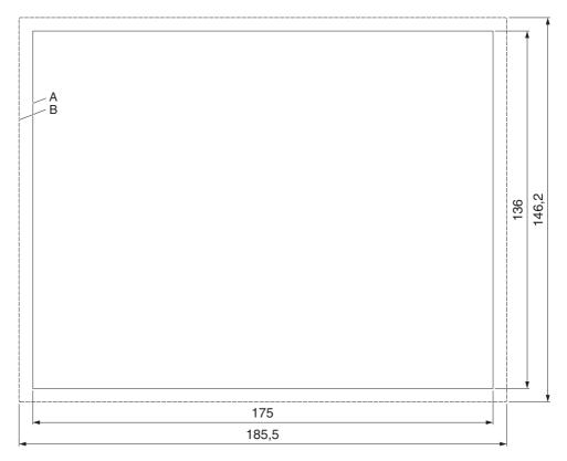
Figure 2-9 Mounting cutout (dimensions in mm)
