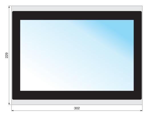
Figure 2-5 Front panel (dimensions in mm)
