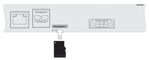
Figure 4-3 Inserting the memory card
