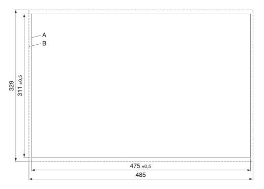
Figure 2-13 Mounting cutout (dimensions in mm)
