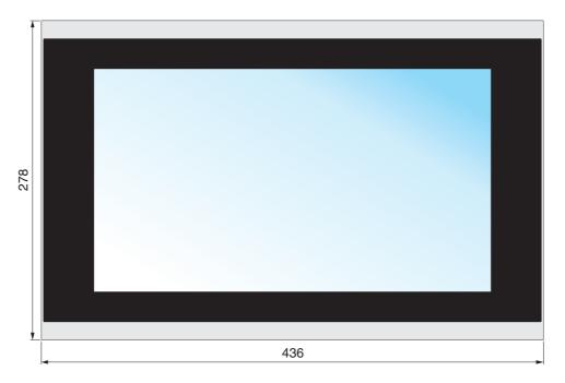
Figure 2-6 Front panel (dimensions in mm)
