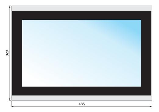
Figure 2-7 Front panel (dimensions in mm)
