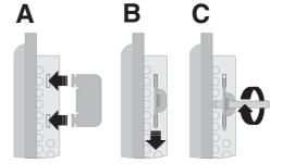
Figure 2-1 Mounting the device using a mounting bracket
