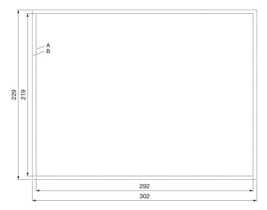
Figure 2-11 Mounting cutout (dimensions in mm)
