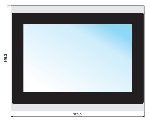
Figure 2-3 Front panel (dimensions in mm)
