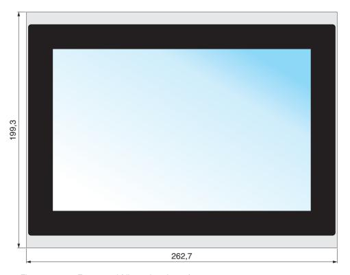
Figure 2-4 Front panel (dimensions in mm)
