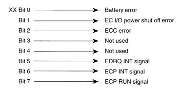
If an alarm occurs, a hexadecimal number is displayed. If "\$C1" is displayed, for example, first convert this "\$C1" into bits.
