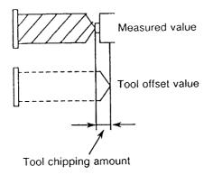
The tool broken alarm occurs if: Broken judgment value < Tool chipping amount (default: 0.1 mm)
