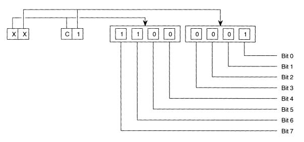
After the conversion, it is known that Bit0, Bit6, and Bit7 are ON. See the information above and you will find that these error codes correspond to "battery error", "ECP INT signal", and "ECP RUN signal", respectively.
