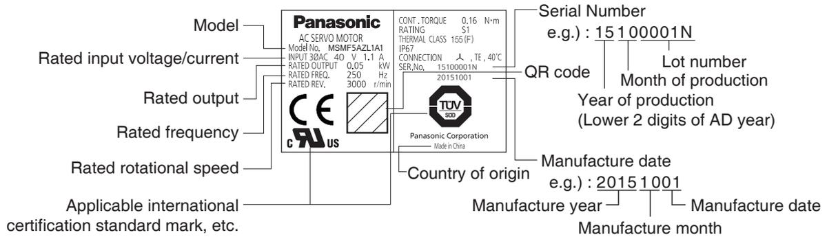
The range of the lot number in serial number is 1 to 33999, but on the nameplate it is written in 4 digits in the following format. In the four digits alphabet, "I" (eye) and "O" (o) are not used.
