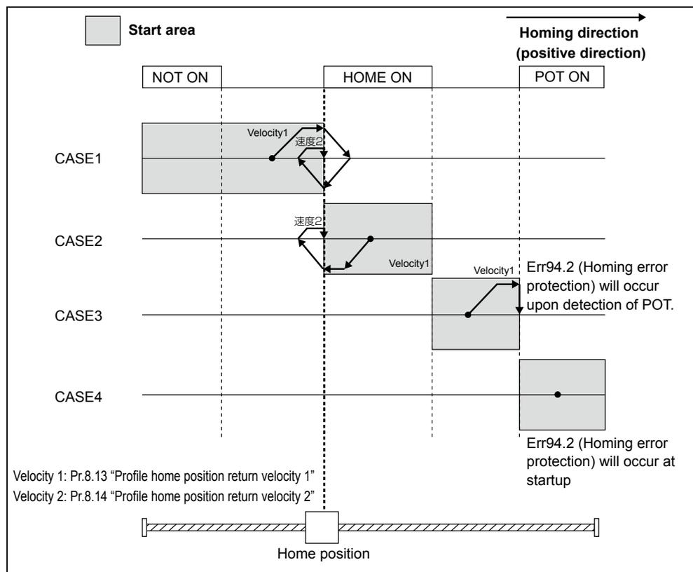
Example: Pr8.12 = 0 (Positive direction trigger signal detection)—homing is started at a position more negative than HOME sensor.
