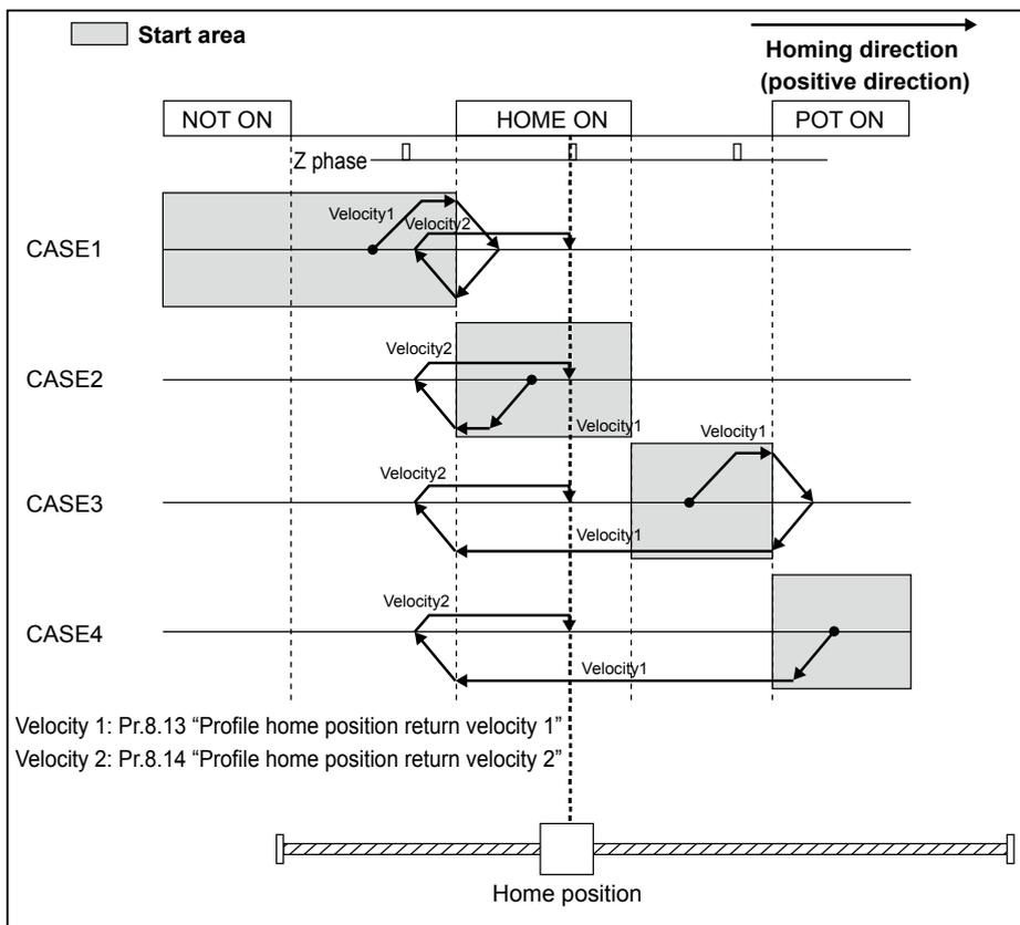
Example: Pr8.12 = 0 (Positive direction trigger signal detection)—homing is started at a position more negative than HOME sensor.
