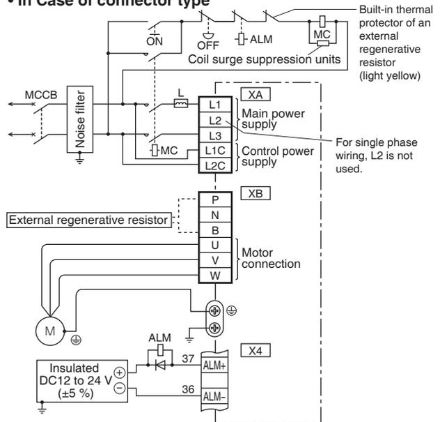
**Note** The external regenerative resistor can be built to A, B-frame.
