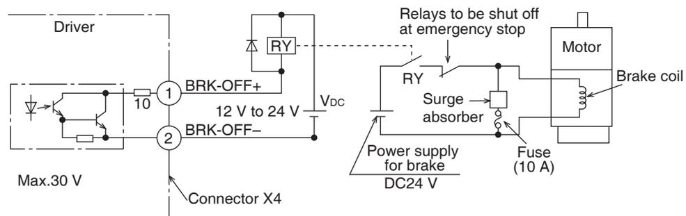
The External brake release signal can be assigned by default setting of SO1(X4:1, 2 Pin).
