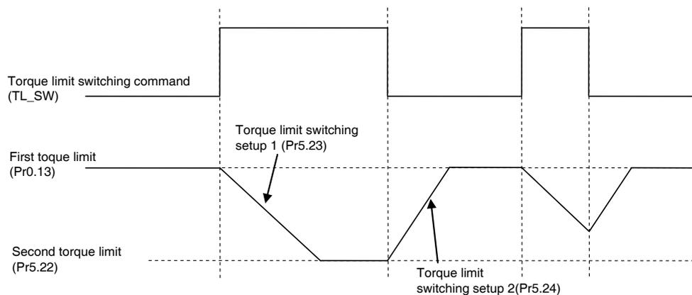
Note) When the first torque limit (Pr0.13) and the second torque limit (Pr5.22) is changed from the setup support software PANATERM or RTEX communication, the change rate setting is ignored and the torque limit value after the change is immediately applied. The change rate setting becomes effective only at the time of switching by the torque limit switching command (TL\_SW).
