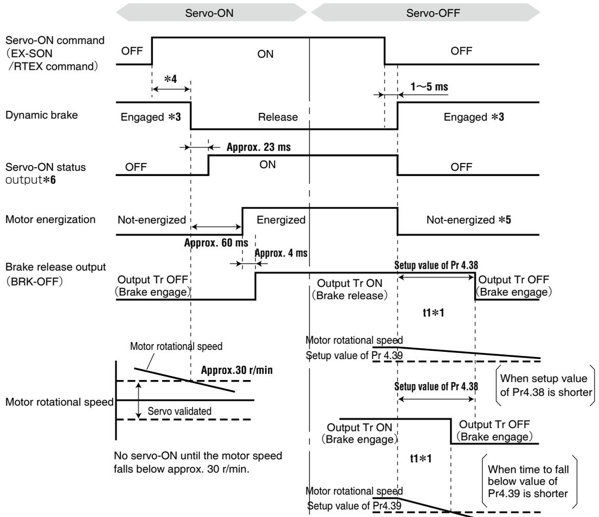
**Caution** ⚙️ \*1  $t1$  will be a shorter time of either the setup value of Pr 4.38 “Mechanical brake action at running setup” or elapsing time for the motor speed to fall below Pr 4.39 “Brake release speed setup”.
