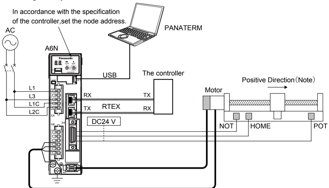
Note : Set the CCW or CW in positive direction by the Pr0.00.
