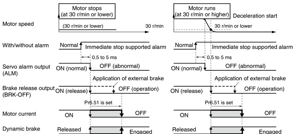
**Note** In the event that the drop prevention function is enabled when alarm is generated, set Pr5.10 "Sequence at alarm" to 4, Pr6.10 "Function expansion setting" bit 10 to "1," and a value longer than the time when brake release output (BRK-OFF) is turned OFF and external brake actually operates to Pr6.51 "Immediate stop end wait time."
