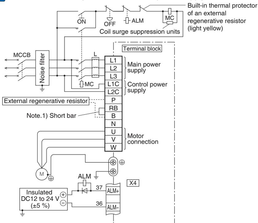
**Note** The regenerative resistor is built into E-frame or can use external regenerative resistor.
