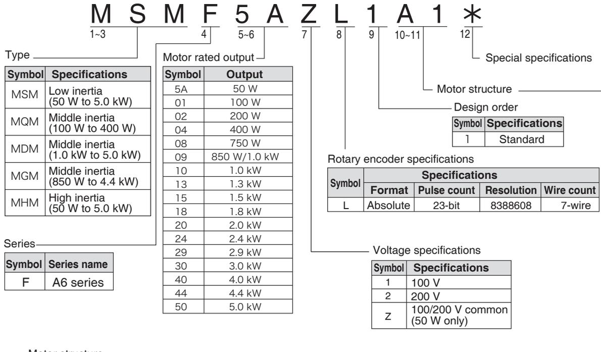
Motor structure \_\_\_\_\_
