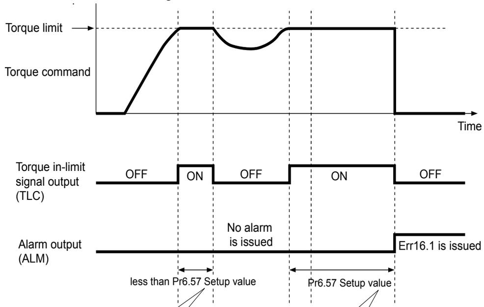
Err16.1 does not occur when the torque saturation condition does not continue for the time set for Pr6.57.
