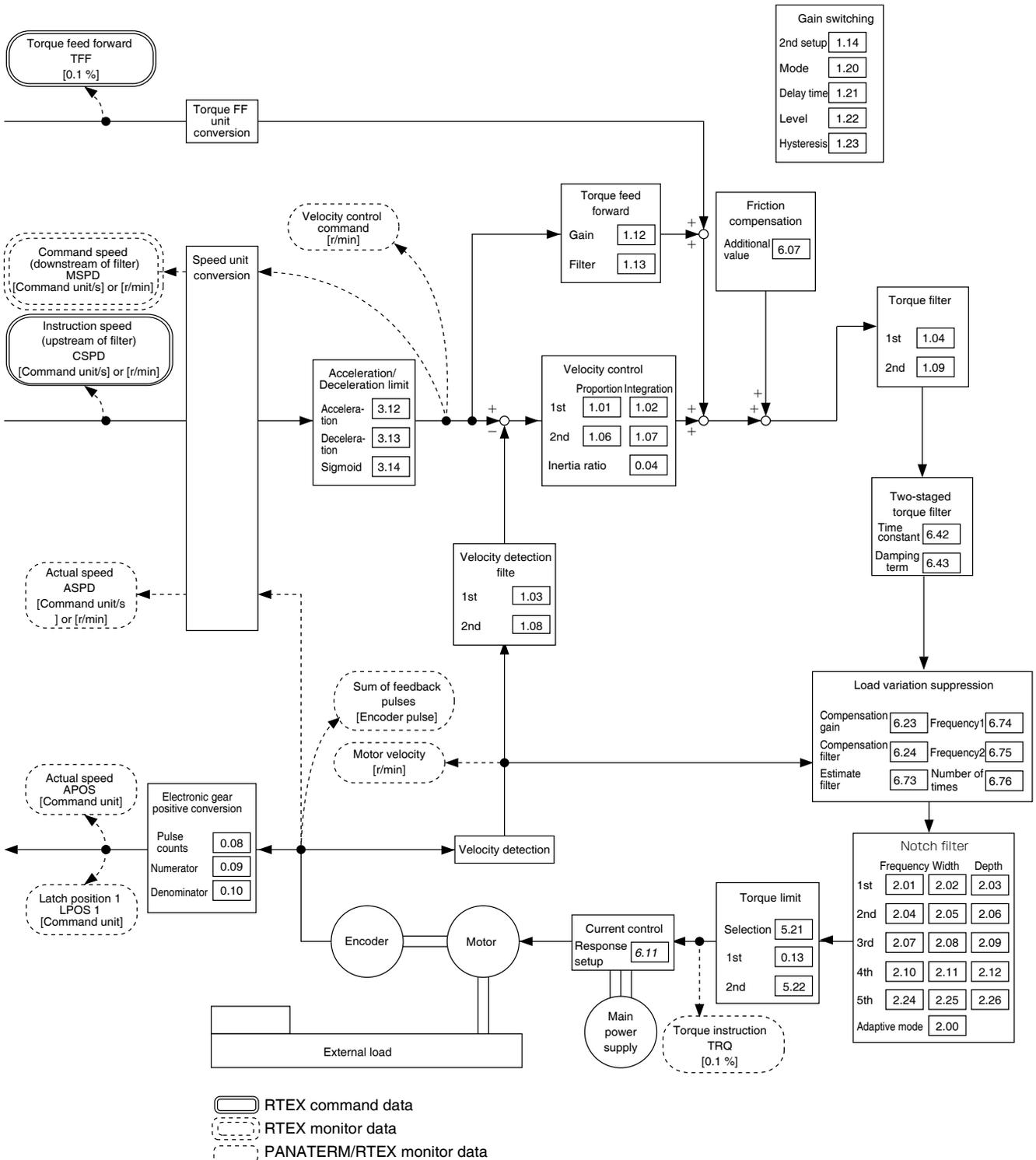
\*1 When performing Frequency characteristic analysis (speed close loop characteristic, Torque speed(Vertical)) from the PANATERM, the driver switches to velocity control mode internally.
