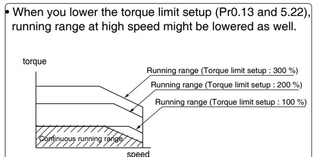
•Note that the motor characteristics may vary due to the existence of oil seal or brake.
