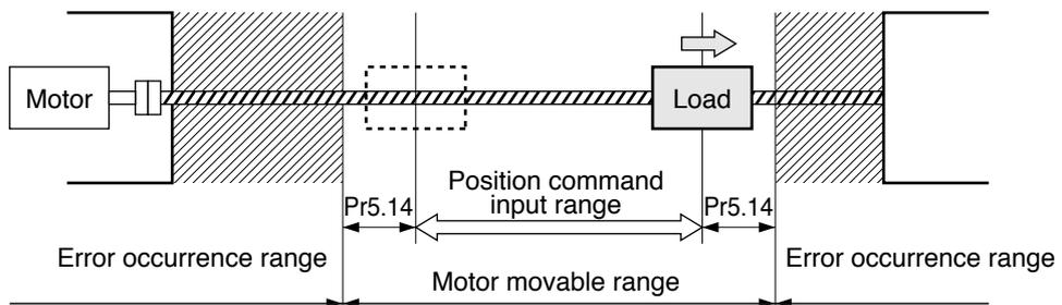
(3) When the load moves to the left (at Servo-ON),
