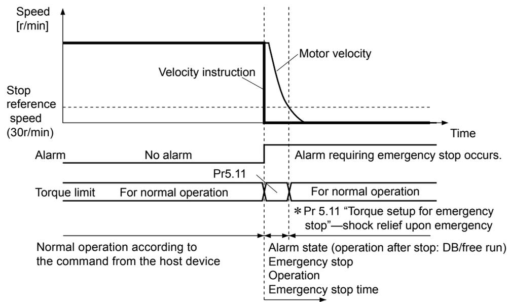
After occurrence of an alarm requiring emergency stop: when the speed has not dropped down to 30 r/min after the elapse of time set by Pr 6.14 "Emergency stop time at alarm", the system generates the alarm. The system also enters the alarm state if an alarm that does not require emergency stop occurs in the driver during the sequence of the emergency stop.
