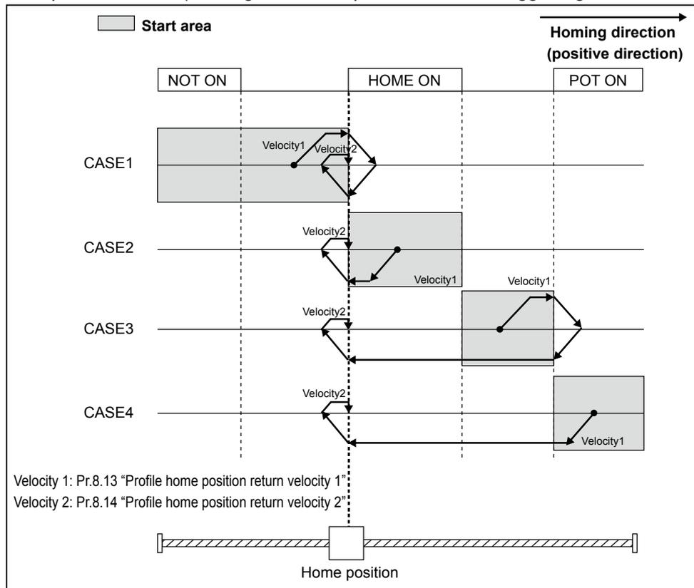
Example: Pr8.12 = 0 (Positive direction trigger signal detection)—homing is started at a position more negative than HOME sensor.
