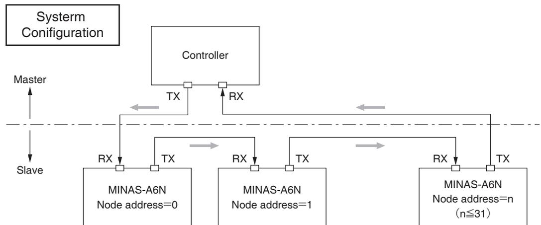
Node address is the ID (MAC-ID) used to identify the slave on the network, and set up with the rotary switch (RSW) on the front panel.
