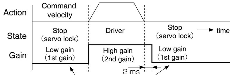
After the end of position command 2s to reduce the gain for vibration suppression.
