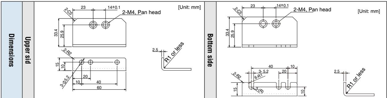
**Caution** For E, F-frame, you can make a front end and back end mounting by changing the mounting direction of L-shape bracket (attachment).
