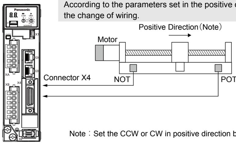
Note : Set the CCW or CW in positive direction by the Pr0.00.
