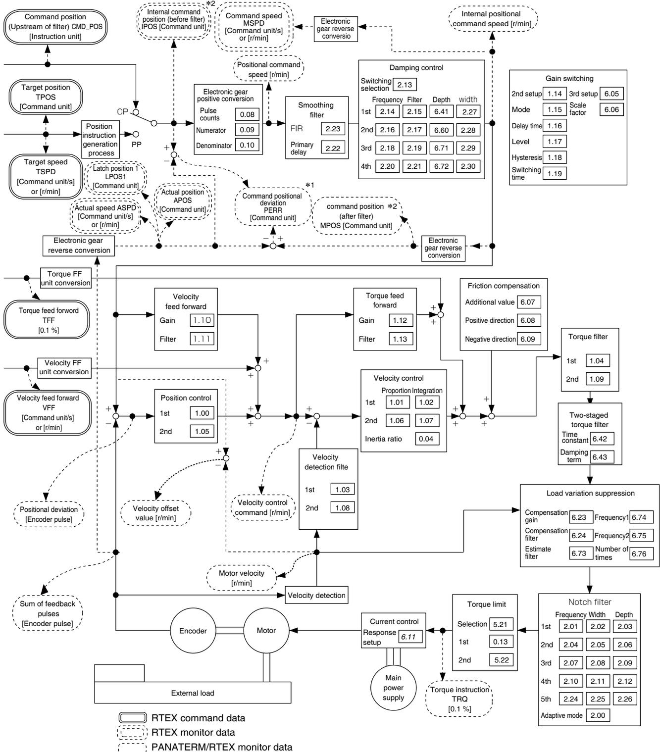
\*1 The computation reference for the command positional deviation [command unit] can be changed by bit14 for Pr7.23 "RTEX function extended setup 2".
