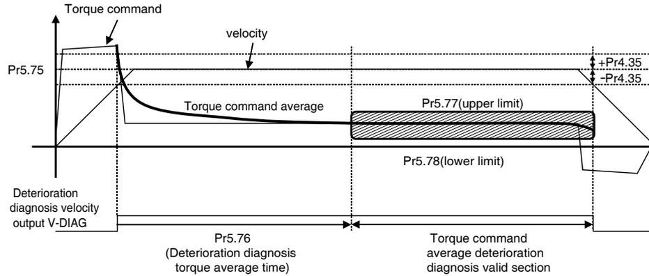
ii) Legend for torque command average deterioration diagnosis warning occurred.
