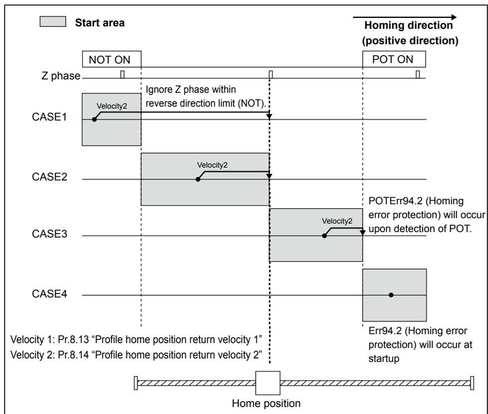
Example: Pr8.12 = 0 (Positive direction trigger signal detection)—homing is started at a position more negative than Z phase.
