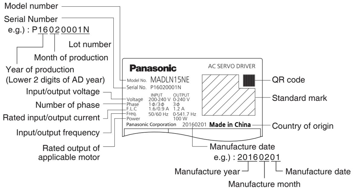
The range of the lot number in serial number is 1 to 33999, but on the nameplate it is written in 4 digits in the following format. In the four digits alphabet, "I" (eye) and "O" (o) are not used.
