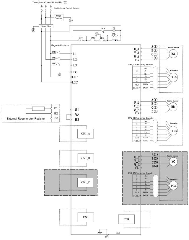
Connect Shield to Connector Shell
