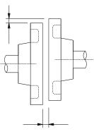
Measure this distance at four different positions in the circumference. The difference between the maximum and minimum measurements must be 0.03mm or less.(Turn together with couplings.)
