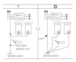
If a noise filter is located inside a control panel, connect the noise filter ground wire and the ground wires from other devices inside the control panel to the ground plate for the control panel first, then ground these wires.
