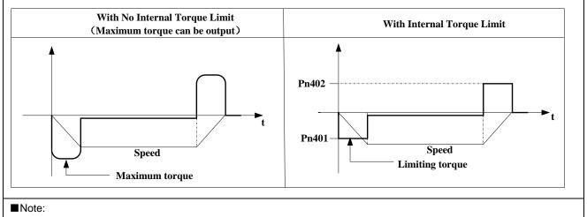
Too small a torque limit setting will result in insufficient torque during acceleration and deceleration.
