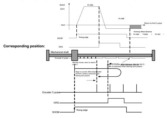
After hitting the origin signal ORG, the motor will find C-pulse directly; the figure is shown as below:
