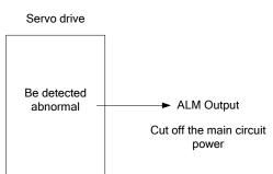
Normally, the external circuit consists of /ALM should be able to switch off the power of servo drive.
