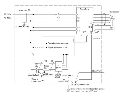
•For ground wires connected to the ground plate, use a thick wire with a thickness of at least 3.5 mm<sup>2</sup> (preferably, plain stitch cooper wire)
