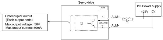
An external +24V I/O power supply is required since there is no +24V power source available inside the servo drive. Output  $\rightarrow$  ALM+CN1\_A/B/C-4 Servo alarm output
