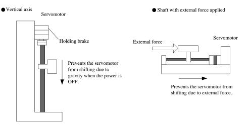
1. The servomotor with the built in brake, is a de-energization brake. It is used to hold the servomotor and cannot be used as a braking purposes. Use the holding brake only to hold a stopped servomotor.
