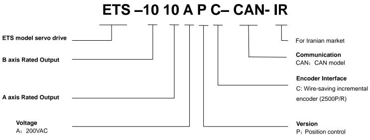
Notes: Each axis of ETS-IR servo drive equips  $50W_100W_200W_400W_750W_1.0kW$  servo motor, and assures three times overload capacity.
