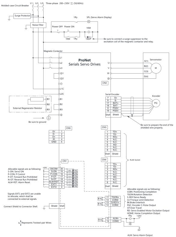
Photocoupler Output: Maximum Operating Voltage: DC30V Maximum Output Current: DC50mA
