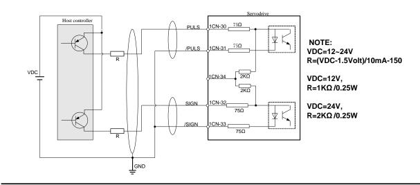
**Note:** When the host controller is applied by open-collector signal output, the input signal noise margin lowers. When a position error caused by the noise occurs, set the parameter Pn006.3.
