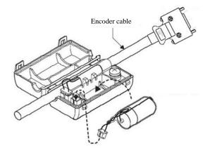
C.Cover the shell of the battery case.
