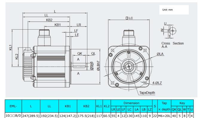
Note: The dimensions in parentheses are for servo motors with holding brake.
