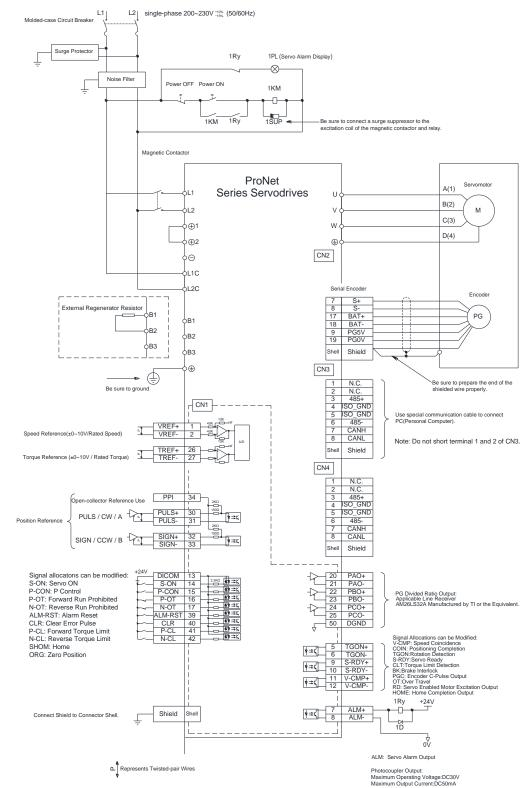
The standard wiring example of ProNet-DDMG servo drives is as shown in the following figure.
