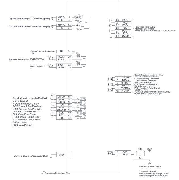
The I/O signal connections diagram of the ProNet-DDMG servo drives is as shown in the following figure.
