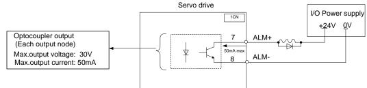
An external +24V I/O power supply is required since there is no +24V power source available inside the servo drive. Output  $\rightarrow$  ALM+ 1CN- 7 Servo alarm output Output  $\rightarrow$  ALM- 1CN- 8 Servo alarm output uses grounding signal
