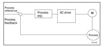
Fig. 73 Closed loop PID control
