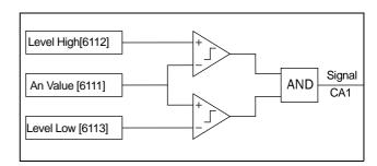
Fig. 94 Analogue comparator type "Window"
