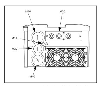
Fig. 9 CDU 48/52: Model 026 to 046 (C), with cable entry/outlets on short side
