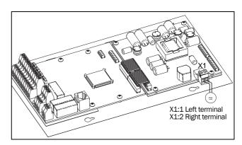
Fig. 112 Connection of standby supply option .
