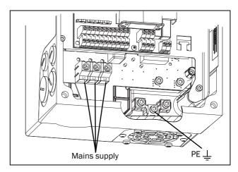
Fig. 10 Mains connections, CDU 008-018 with side cable entry/outlet.
