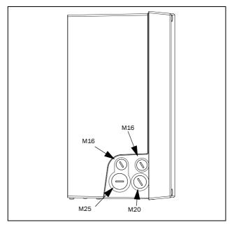
Fig. 6 CDU 48/52: Model 008 to 018 (B) with side cable entry/outlets.
