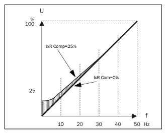
Fig. 70 IxR Comp at Linear V/Hz curve
