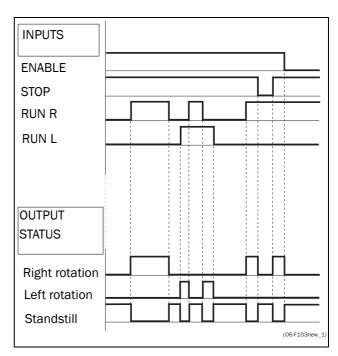
Fig. 26 Input and output status for level-control
