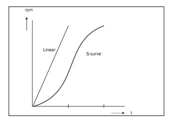
Fig. 63 Shape of acceleration ramp
