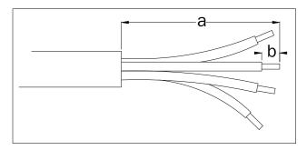
Fig. 14 Stripping lengths for cables
