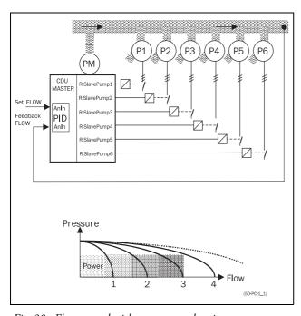
Fig. 30 Flow control with pump control option
