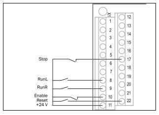
Fig. 25 Example of wiring for Run/Stop/Enable/Reset inputs
