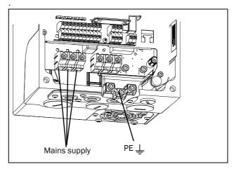
Fig. 11 Mains connections, CDU 008-018 with cable entry/outlet on short side.
