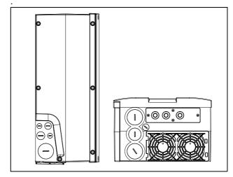
Fig. 4 CDU 48/52 Model 026 to 046, frame size C with cable inlet from long side (standard) or short side
