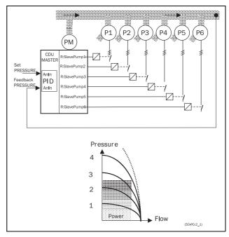
Fig. 31 Pressure control with pump control option
