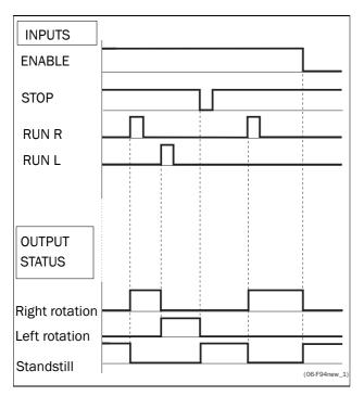
Fig. 27 Input and output status for edge-control
