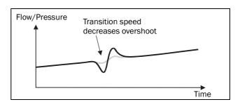
Fig. 82 Effect of transition speed
