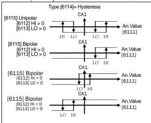
Fig. 97 Principle functionality of comparator features for "Type [6114] = Hysteresis" and "Polar [6115]".
