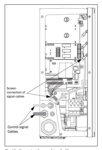
Fig. 19 Connecting the control signal cables to CDU 026 - 046
