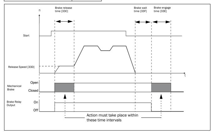
Fig. 65 Brake Output functions
