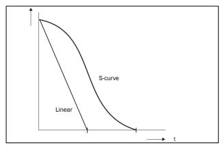
Fig. 64 Shape of deceleration ramp
