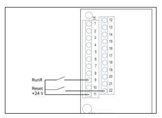
Fig. 23 Default setting Run/Reset commands
