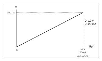
Fig. 88 Normal full-scale configuration
