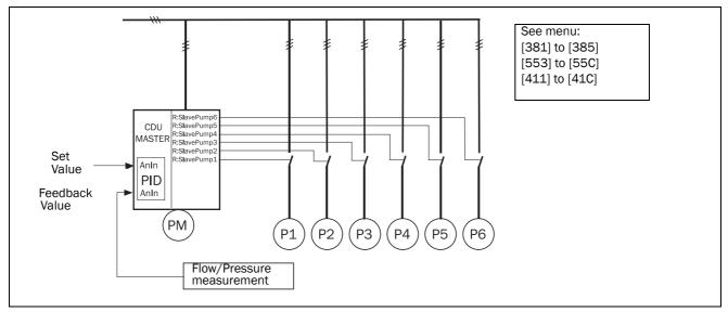
Fig. 36 PID control
