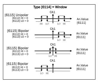
Fig. 98 Principle functionality of comparator features for "Type [6114] = Window" and "Polar [6115]".
