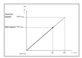
Fig. 60 Acceleration time and maximum speed
