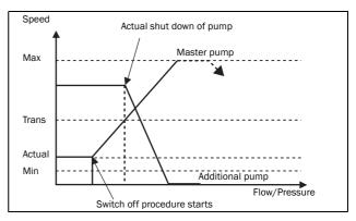
Fig. 83 Transition speed stop
