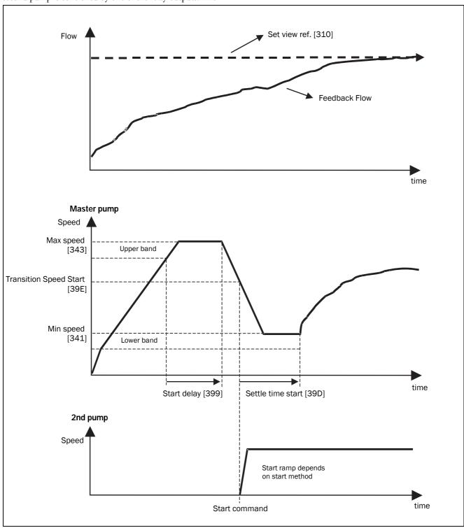
Fig. 37 Time sequence starting an additional pump
