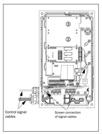
Fig. 18 Connecting the control signal cables to CDU 008 - 018
