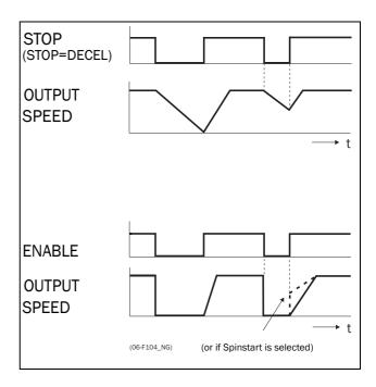
Fig. 24 Functionality of the Stop and Enable input
