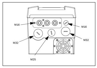
Fig. 7 CDU 48/52: Model 008to 018 (B) with cable entry/outlets on short side.
