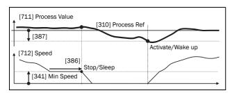
Fig. 74 PID Stop/sleep with normal PID
