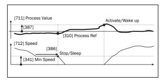
Fig. 75 PID Stop/sleep with inverted PID
