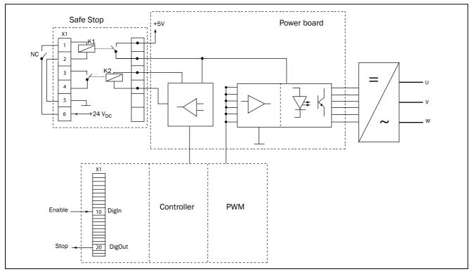
Fig. 115 Safe Stop connection
