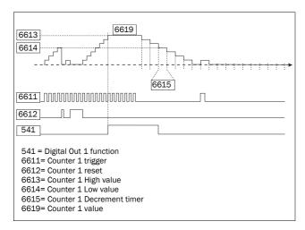
Fig. 102 Counters, operating principle.
