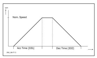
Fig. 61 Acceleration and deceleration times
