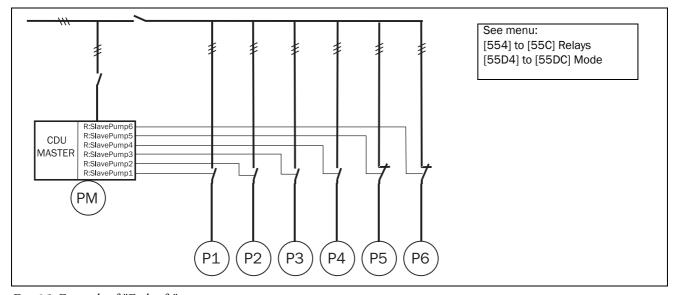
Fig. 35 Example of "Fail safe" operation
