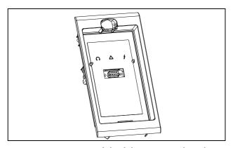
Fig. 52 RS232 connector behind the HCP control panel (Optional)
