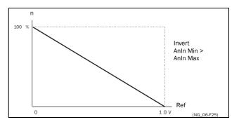
Fig. 90 Inverted reference
