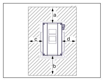
Fig. 5 Variable speed drive mounting models 008 to 046
