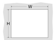
For the installation into a operating tableau and control cabinet fronts, the Touch Panel requires the following front plate cutting:
