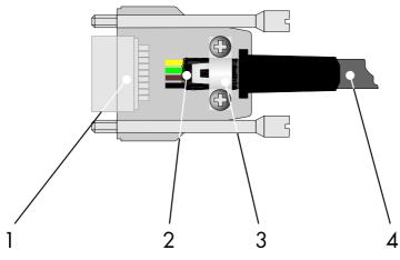
Figure 4-16 Shielding D-SUB connectors
