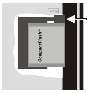
Figure 4-15 Ejecting the memory card
