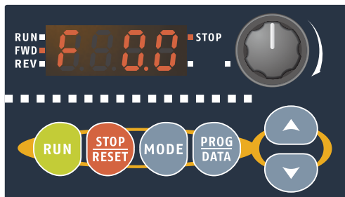
When power is ON, it will be displayed „F0.0“ and LED „STOP“ and „FWD“ should light up
