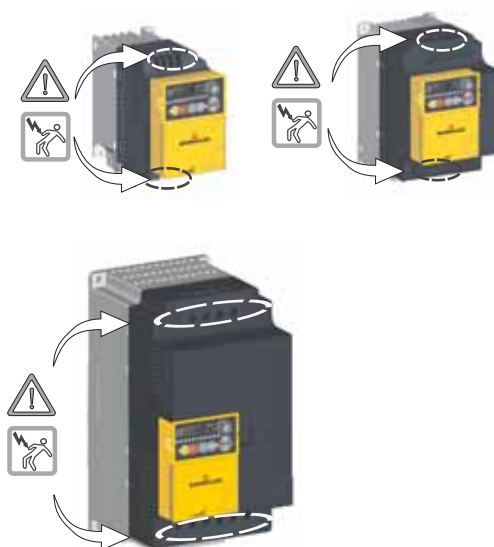
Figure 21: Danger areas at the electrical installation
