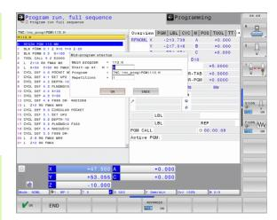
▶ Go to the first block of the current program to start a block scan: Enter GOTO "0"
