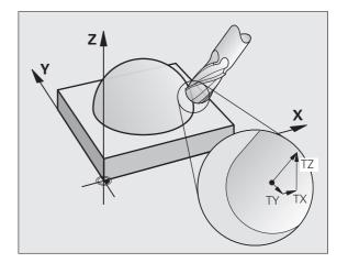
Example: Block format with surface-normal vectors without tool orientation
