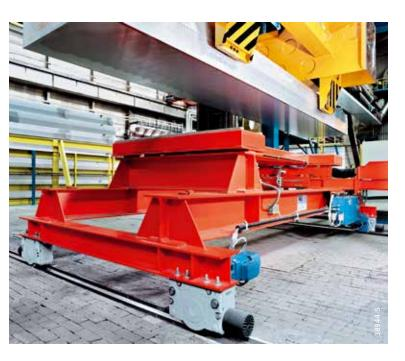
Four-wheel trolley controlled by a frequency inverter for smoothly moving blocks of aluminium
