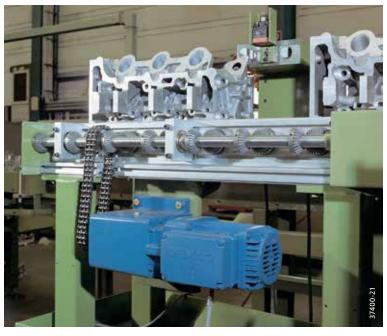
Roller conveyor operating at precisely adjusted speed
