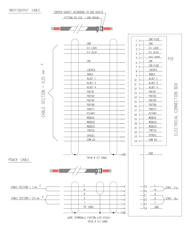
NB. -On CM1 and CM2 connections there are F1 and F2 protection fuses (see wiring diagram sheet 8) -For first connection and start-up please use P10/7 and P10/1 pins,and than, after positive test, shift the connections on P10/6 and P10/2 pins
