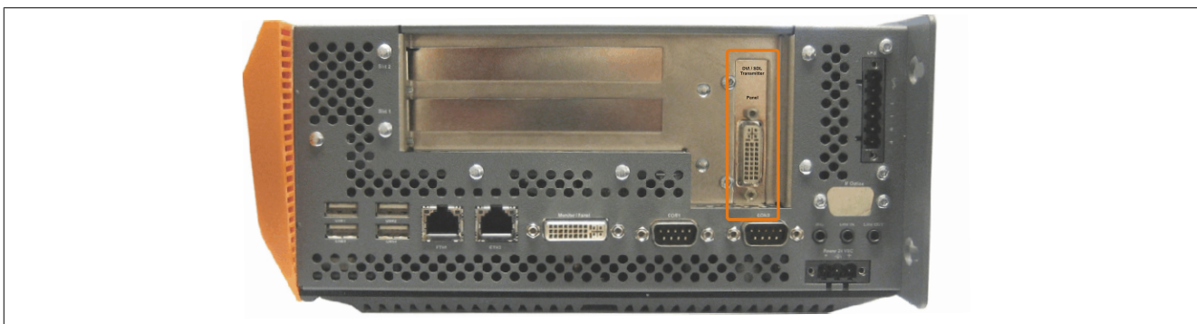
Figure 80: 5PC810.SX02-00 - Installation example in system unit
