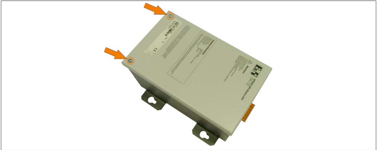
Figure 279: Removing the cover for the battery unit
