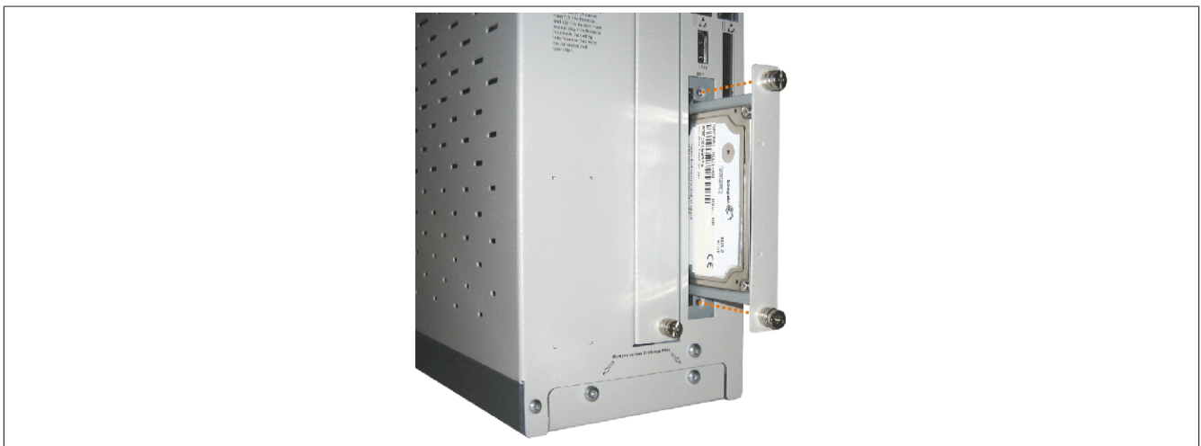
Figure 235: Inserting the compact SATA drive
