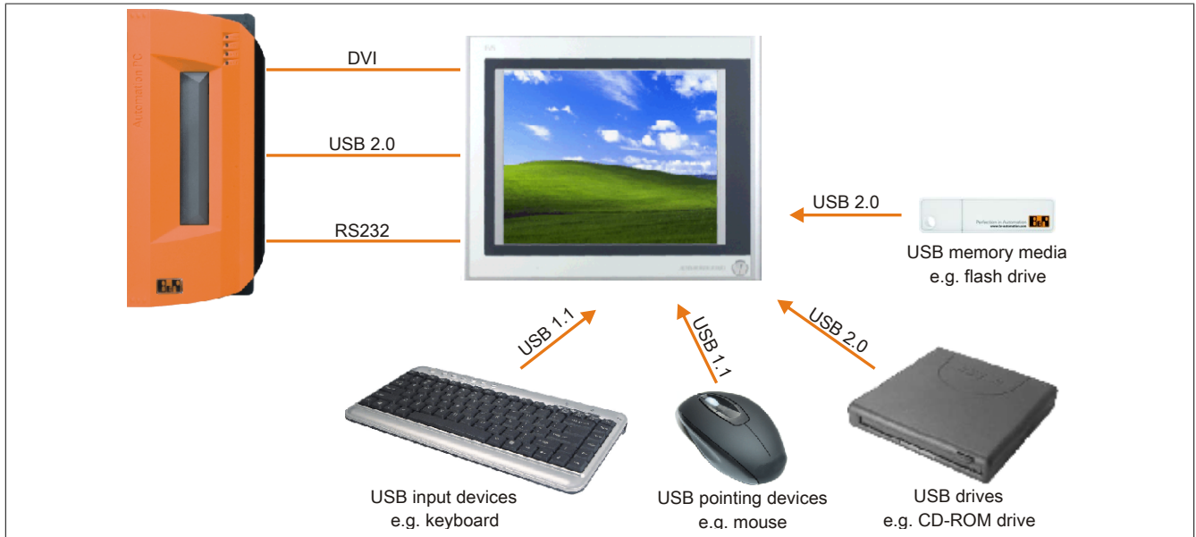
Figure 107: Remote connection of USB peripheral devices on the APC900 via DVI
