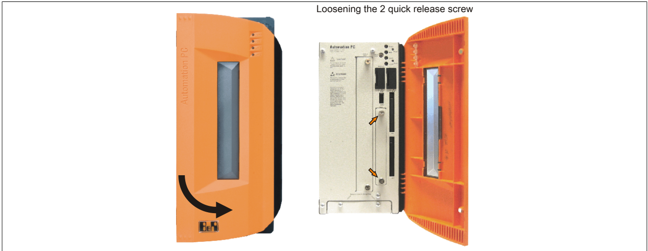
Figure 234: Loosening the quick release screws
