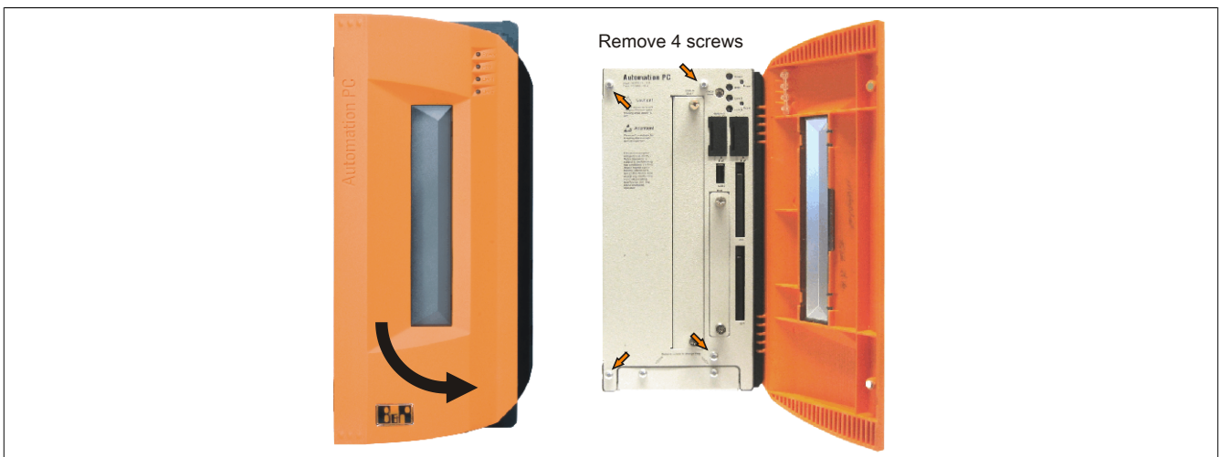
Figure 284: 2-slot APC810 - Installing the side cover
