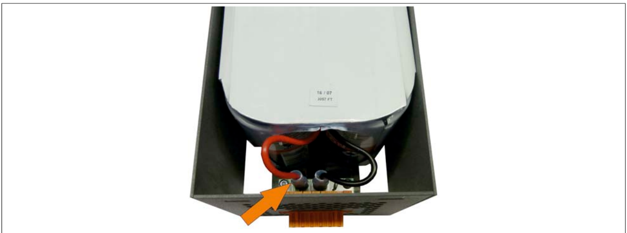
Figure 280: Disconnecting the cable
