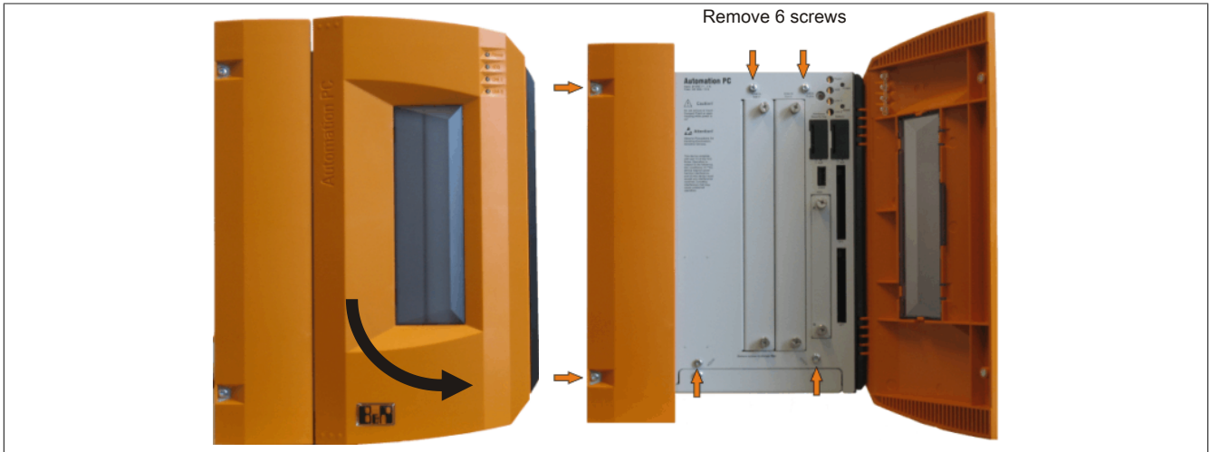
Figure 285: 5-slot APC810 - Installing the side cover
