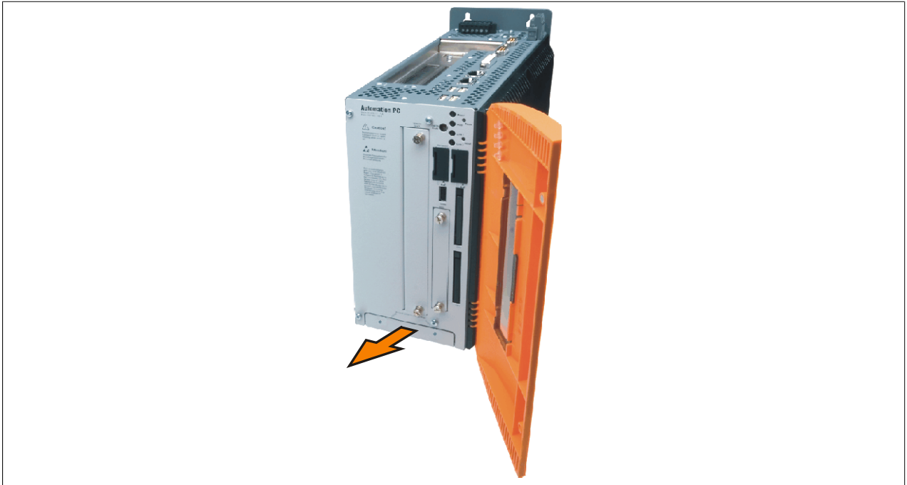
Figure 241: Removing the fan kit insert
