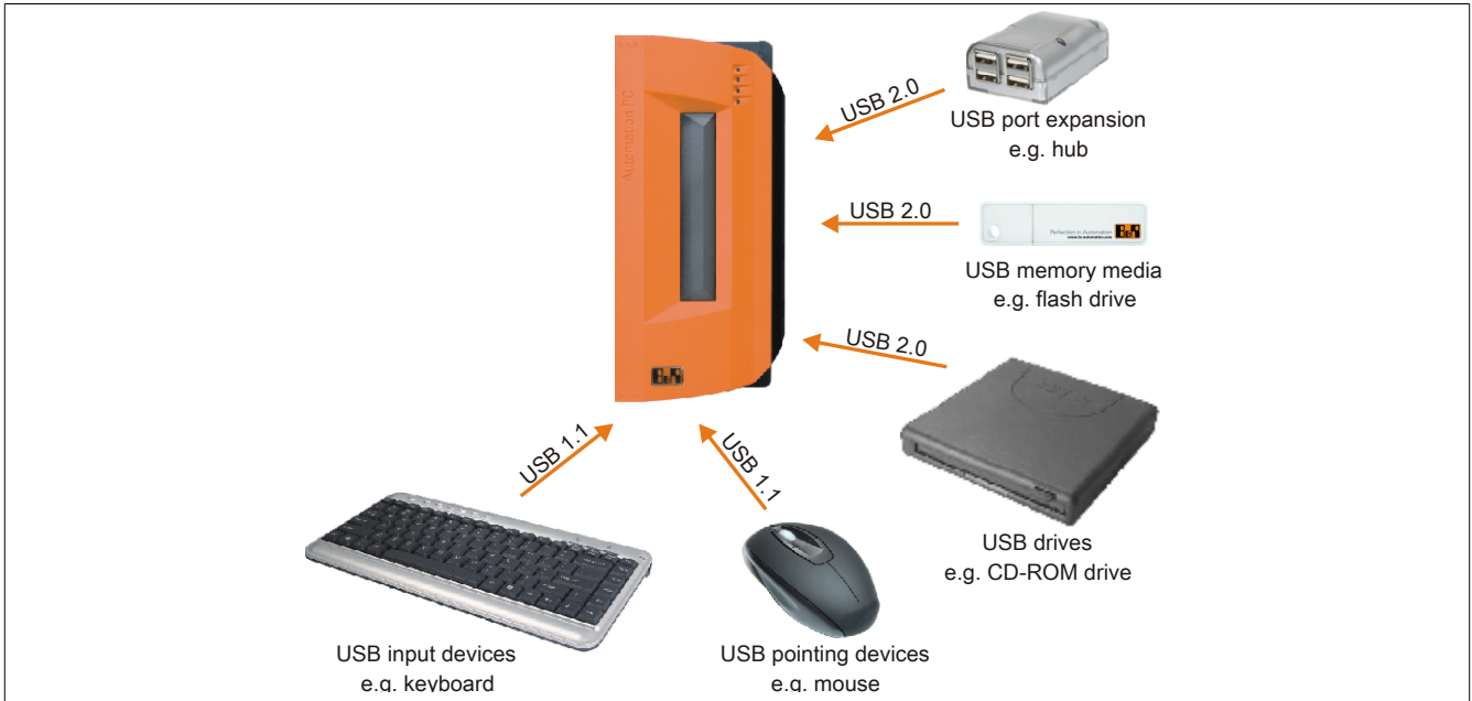
Figure 106: Local connection of USB peripheral devices on the APC810
