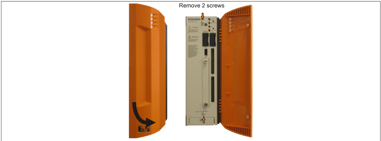
Figure 283: 1-slot APC810 - Installing the side cover
