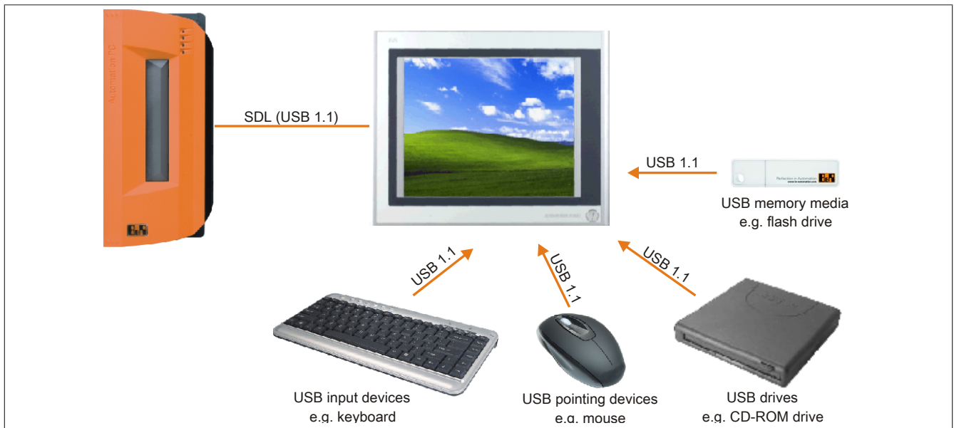
Figure 108: Remote connection of USB peripheral devices on the APC800/900 via SDL
