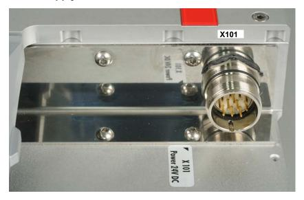
The power supply connection of the Industrial PC and the connection with the UPS (optional) is established via the power supply socket (**X101**).
