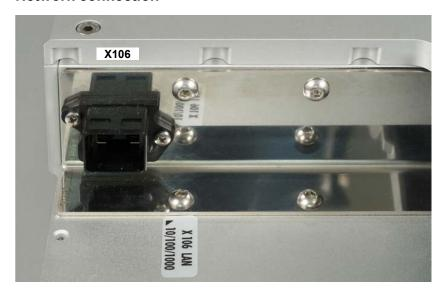
The Ethernet-interface with RJ-45-connector (**X106**) allows the PC to be connected to a network (LAN). In the basic configuration a Gigabit-port is available.
