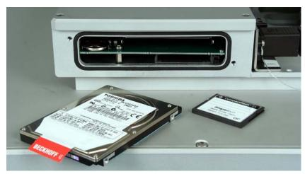
The hard-disk drive and the memory card can now be pulled out. Here, changing the lithium battery is also possible.
