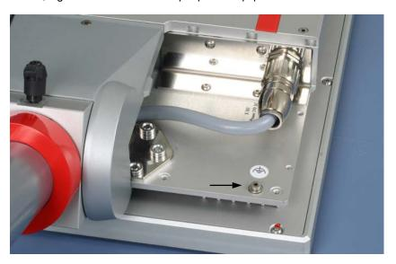
The picture shows the earthing connection in the wiring area of the PC (see arrow). The earthing cable is laid through the support arm.
