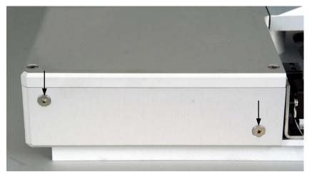
After unscrewing the two Allen screws (see arrows) the drive cover can be taken off.
