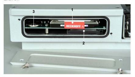
Removing the drive cover allows access to the IDE-hard-disk (1) (optional), the Compact-Flash-memory card (2) and the lithium battery of the system clock (3).
