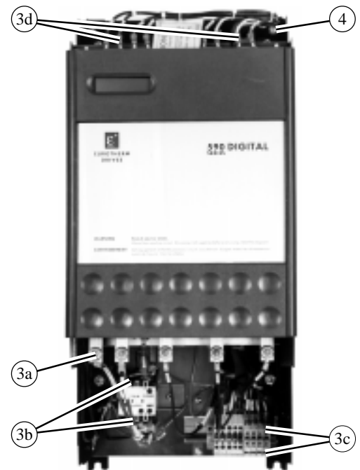
Figure 6.3 - 590 DRV with Lower Cover Removed
