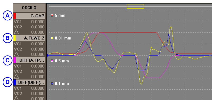
Speed and acceleration profile without overshooting the gap.
