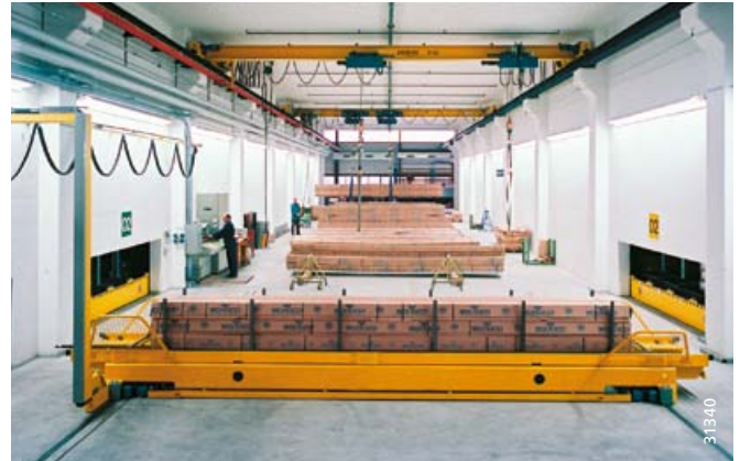
The load – positioned with millimetre accuracy – can be fed through the openings in the walls
