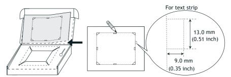
3. Secure the operator panel in position, using all the fastening holes and the provided brackets and screws:
