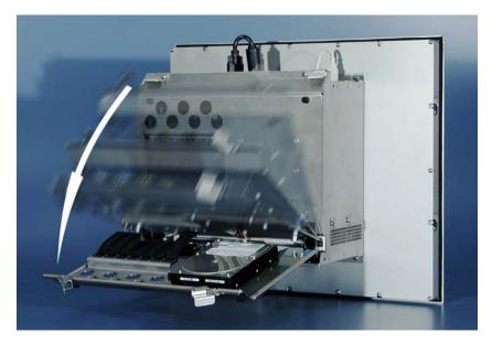
The chassis can now simply be folded out backwards, thus providing access to the hard drive, processor, memory and plug-in cards.
