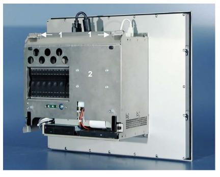
Unfasten the two securing levers (1) that hold the fold-out inner chassis (2).
