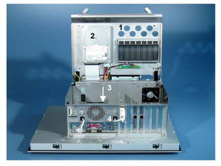
When the inner chassis (1) has been folded out of the way with the hard drive (2), a 7-slot ATX motherboard (3) is found. The connections are accessible from outside (4).
