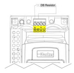
Figure 5.1 External Braking Resistor
