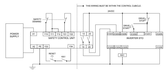
**Note:** On power-up, the safety control unit outputs are OPEN; thus the STO state is requested of the inverter. The latter responds by energising KA1 if both channels are active and healthy. KA1 is used as a self-check for the reset cycle of the safety control unit. If a reset cannot be achieved due to KA1 being de-energised, a fault may be present and must be resolved by the user before relying on the STO function. See Fault Operation on page 6-14.
