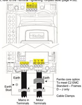
Frame K - no DB+ connect resistor between DC+ & DB)
