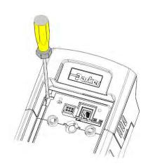
Disconnecting the Ethernet Cable - AC30V
