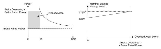
The **Braking** feature also provides a control signal that is used by the **Slew Rate** limit feature. This causes the setpoint to be temporarily frozen whenever the brake is operating because the dc link voltage exceeds the internal comparison level. This allows the stop rate to be automatically tuned to the characteristics of the load, motor, Drive and brake resistor.
