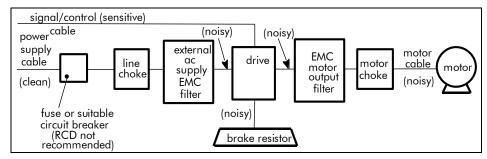
Figure C-2 Cabling Requirements
