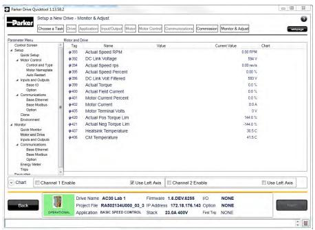
Figure 9-15 Monitor the Drive and fine tune
