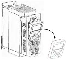
**2.** Undo the screw and slide the control module cover down slightly, then remove.
