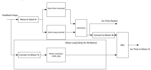
Short Overload: is using 180% of the Heavy Duty rating, for 3s. Long Overload: is using the overload mode selected in **0390 Duty Selection**.
