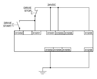
STO inputs X10/01 and X10/03 must be connected to 24VDC with respect to terminals X10/02 or X10/04.
