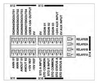
Control Wiring Layout Diagram
