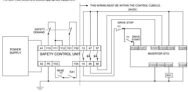
**Note:** On power-up, the Safety Control Unit outputs are OPEN; thus STO is requested of the inverter. This responds by energising KA1 if both channels are active and healthy. KA1 is used as a self-check for the reset cycle of the Safety Control Unit. If a reset cannot be achieved due to KA1 being denergised, a fault may be present and must be resolved by the user before relying on the STO function. See Fault Operation on page 6-14.
