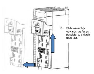
4. Lift assembly away from Power Stack
