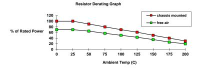
Figure 5.2 Braking Resistor Derating Graph (Metal Clad Resistors)
