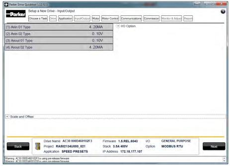
Figure 9-7 Drive I/O setup
