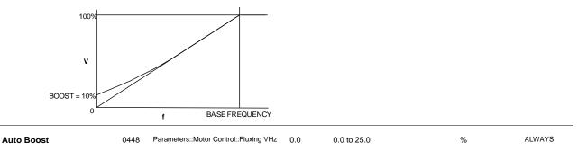
This parameter allows for load dependent stator resistance voltage drop compensation. This correctly fluxes the motor (under load conditions) at low output frequencies, thereby increasing available motor torque. **Auto Boost** can be set in addition to **Fixed Boost**.
