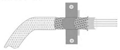
Figure C-1 360 Degree Screened Connection (Motor)
