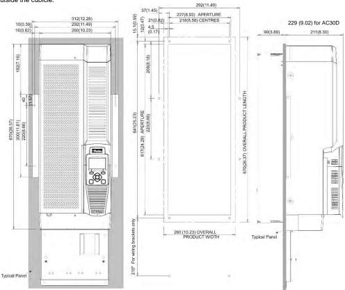
Figure 4-6 Mechanical Dimensions for Through Panel Frame H
