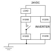
The load is energised and X10/05 is high when STO is in the intended safe STO state.
