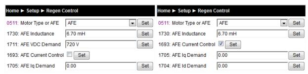
AFE inductance parameter must be set to the value of the total line choke inductance.
