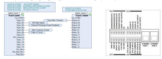
The default macro requires the following electrical wiring diagram for AC30P/AC30D control board. Use of different inputs will need to be accompanied by the appropriate change in the application.
