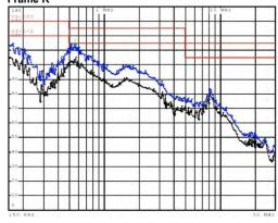
Typical common d.c bus system emissions, for reference (800uH a.c. choke + 890CS supplying 740-4D0012 + 740-4E0023) (Actual system emissions will depend on the details of the specific application.)
