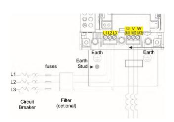
AC Motor Chokes. Only on long cable runs >50m
