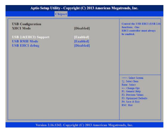
USB 2.0(EHCI) Support Enables or disables the Enhanced Host Controller Interface (USB 2.0), one EHCI controller must always be enabled.
