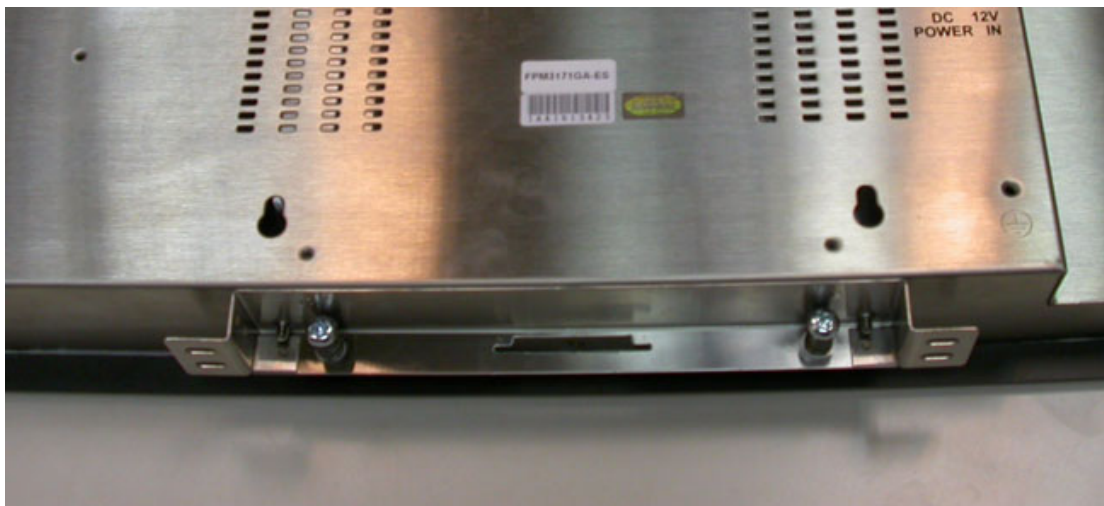
Figure 2.4: Bracket Arranged for Panel Mounting
