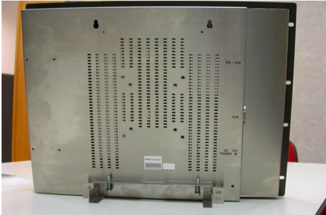
Figure 2.6: FPM-3170 Mounted on Desktop Stand
