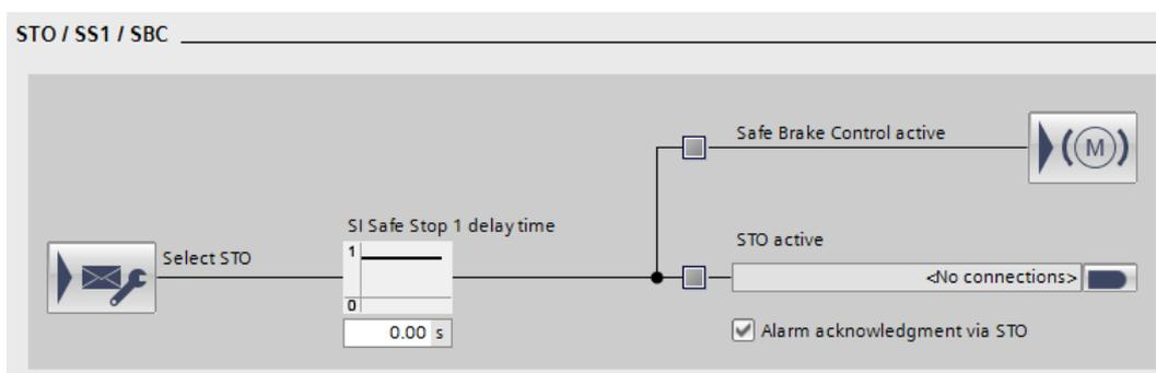
Рисунок 11-8 Safety Integrated Basic Functions STO, SS1, SBC
