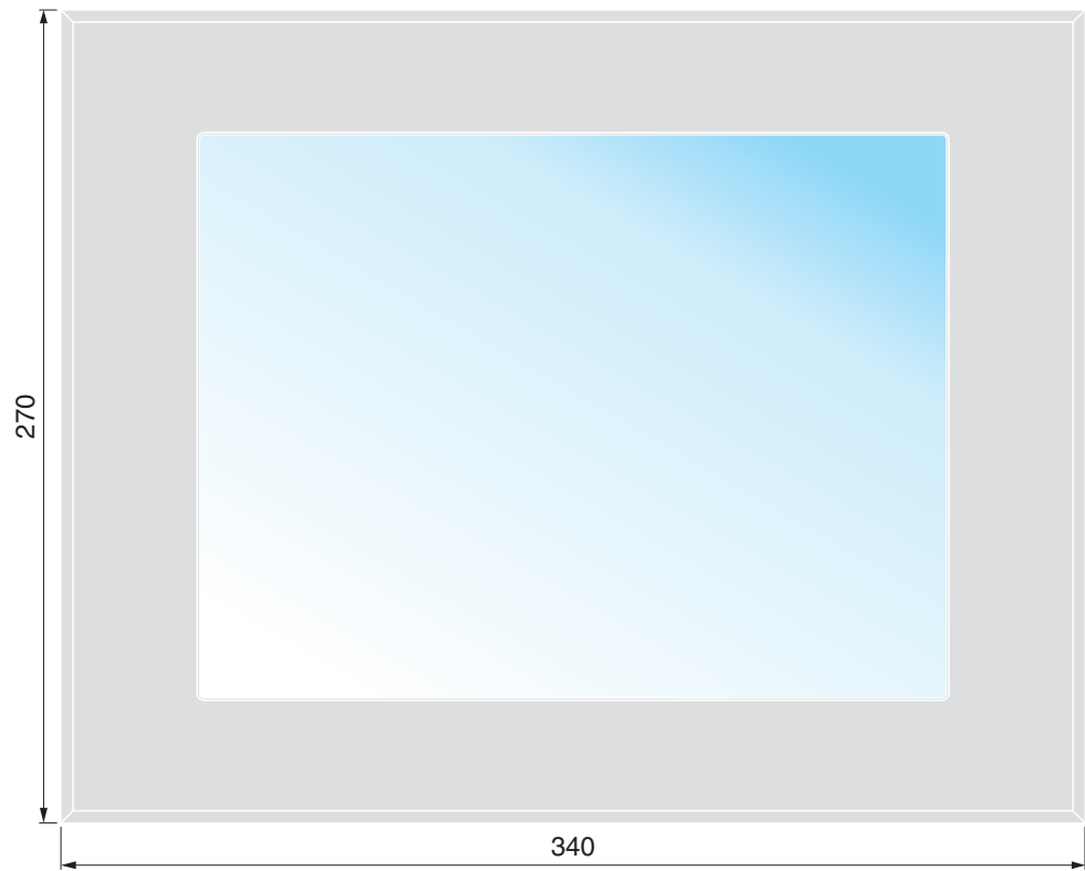
Figure 2-8 Front panel (dimensions in mm)
